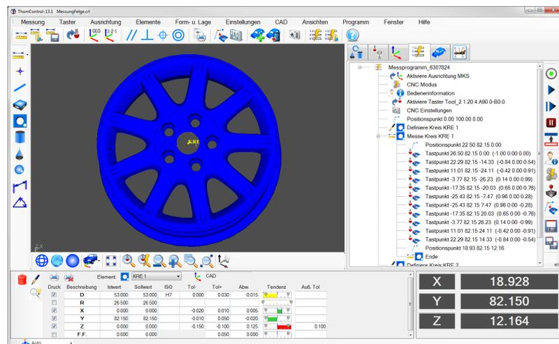
CAD files in IGS and STEP format can be imported. Elements can be selected via the CAD file with a mouse click and automatically measured. The software proposes a measurement strategy and shows the paths graphically. The strategy may be modified as required.
