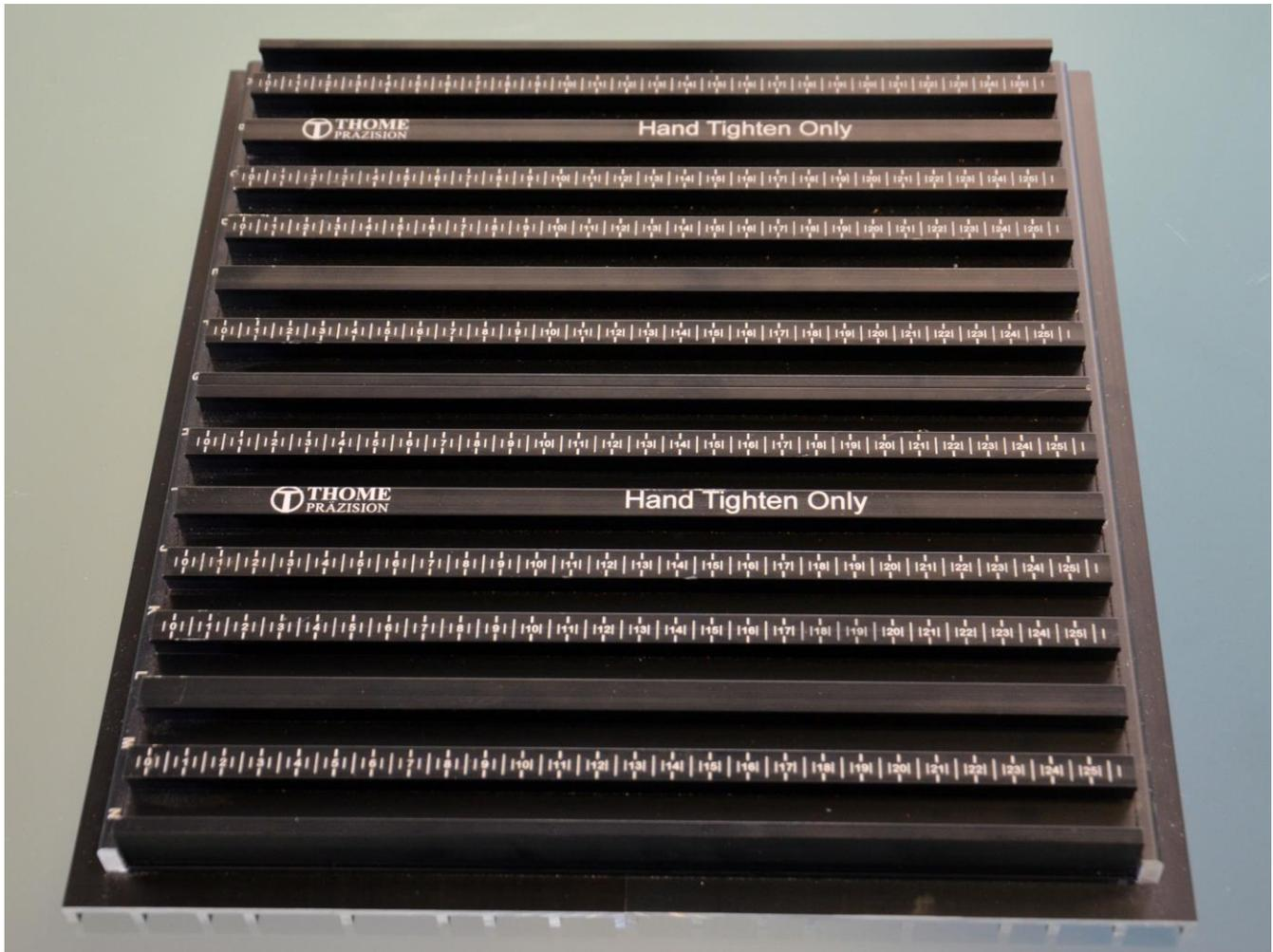
All clamping plates have T-slots and engraved line markings at 25 mm intervals. They serve as an orientation aid when setting up reproducible fixtures.
