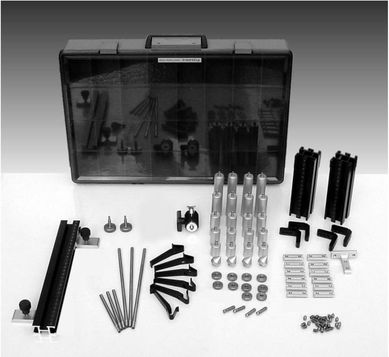
The Kit Standard clamping system is suitable for small to medium-sized workpieces up to a weight of 50kg.
